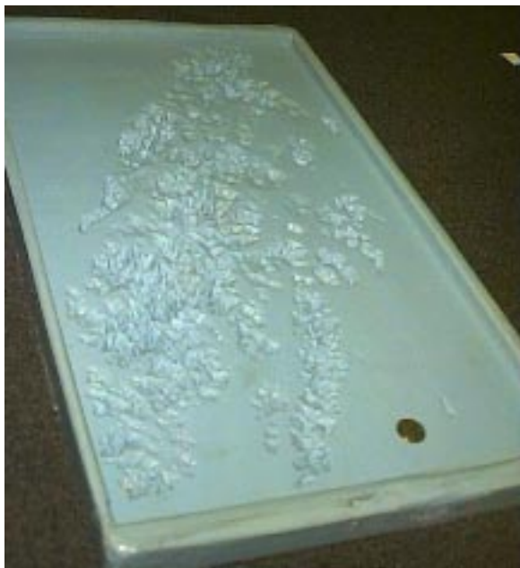
Figure 7: Negative Cast Created from Molding Compound
